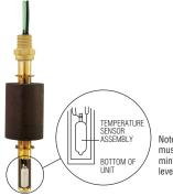
Note: End of unit stem must be submerged a minimum of 2-3/4" for level switch actuation.
