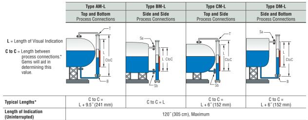
Formula provided is for approximation only. Final dimensions will vary due to connections type, position, cable or junction box location, and specific gravity of process liquid. Gems will confirm final dimensions before manufacturing.
