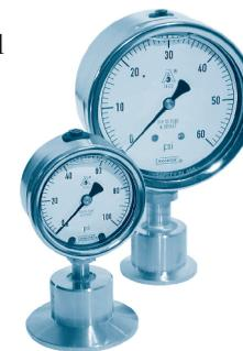
10 Series Heavy-Duty Gauges are available for ranges in vacuum and compound through 600 psi and process temperatures up to 300°F (150°C). 2-1/2" and 4" sizes are available, with 1-1/2" or 2" clamped-style process connections. These gauges feature electropolished 304 stainless steel cases with welded 316L stainless steel sockets and clamped-style process connections. Dry and liquid filled cases are available.
