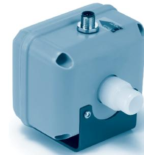
With no metallic parts (100% PVDF body and PVDF carbon fiber-filled electrodes), the meter is corrosion-resistant and compatible with a wide range of chemicals. Accuracy is maintained with conductive fluids (>20 microSiemens) of varying viscosities and densities. The housing is made of sturdy splashproof HDPE plastic.
