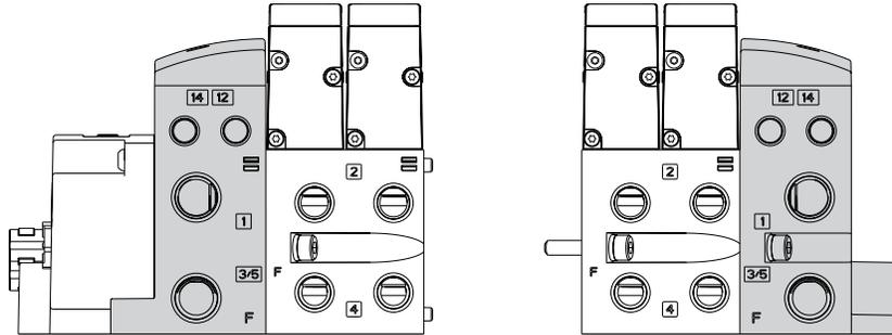
Shaded components are described by the manifold assembly number. The communications module is described by the electronic interface model number designation.
