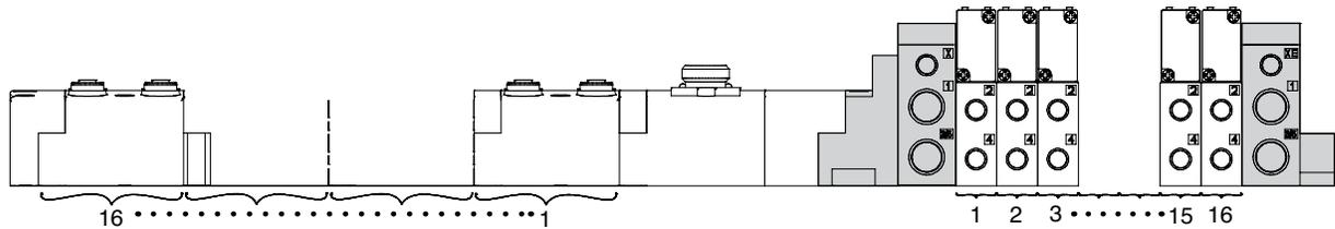
Shaded components are described by the assembly kit (AK) model number (see previous page). The communications module and number of I/O modules are described by the electronic interface (G3) model number designation (see previous page).
